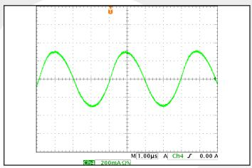
**Figure 9:** Input terminal current ripple, i<sub>C</sub>, at full rated output current and nominal input voltage with SynQor MCOTS filter module (200 mA/div). Bandwidth: 20MHz. See Figure 17.
