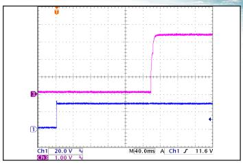
Figure 8: Turn-on transient at full resistive load and zero output capacitance initiated by Vin. ON/OFF Pin previously low. Ch 1: Vin (20V/div). Ch 3: Vout (1V/div).
