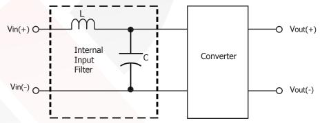
Figure E: Internal Input Filter Diagram
