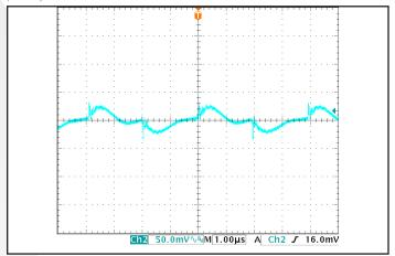
**Figure 10:** Output voltage ripple, Vout, at nominal input voltage and rated load current (50 mV/div). Load capacitance:  $1\mu F$  ceramic capacitor and  $15\mu F$  tantalum capacitor. Bandwidth: 10 MHz. See Figure 17.
