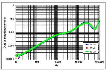
Figure 13: Magnitude of incremental output impedance  $(Z_{out} = v_{out})$ iout) for minimum, nominal, and maximum input voltage at full rated
