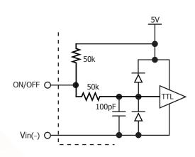
Figure B: Internal ON/OFF pin circuitry
