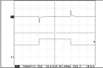
Figure 11: Output voltage response to step-change in load current (50%-75%-50% of Iout(max);  $dI/dt = 0.1 A/\mu s$ ). Load cap:  $1 \mu F$  ceramic and  $15 \mu F$  tantalum capacitors. Ch 1: Vout (100mV/div), Ch 2: Iout (10A/div).
